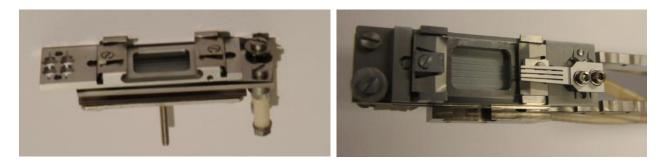
This package is designed to **upgrade the discontinued tungsten wire sample heater S7106**, which was supplied with **Scienta Omicron manipulators**, with the current resistive sample heater solution: The coplanar Porolytic Boron Nitride heater element offers great uniformity, high durability and is easy to replace. It can be operated up to a maximum heating power of 100 W (3 A), allowing typical sample temperatures of up to 1170 K (up to 1100 K with optional  $IN_2$  cooling).
