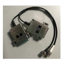
Enables upgrade of early LT-STM instruments with V4 Preamplifier technology (SPM PRE 4E)
