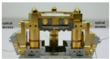
2 optical access points at 90° and 270° with respect to the wobblestick axis. The tilt angle towards the sample face is 25°
