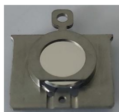
Picture represents test samples in PEEM sample plate D201101-S. Please consider the height of 3 mm of the sample surface with respect to the sample plate.
