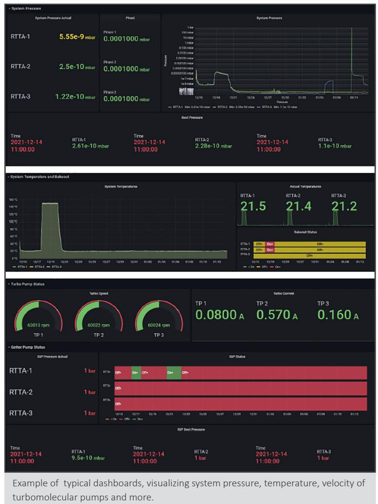
Example of typical dashboards, visualizing system pressure, temperature, velocity of turbomolecular pumps and more.
