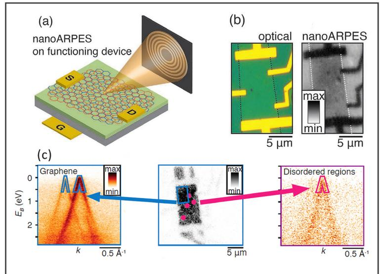
nanoARPES of twisted bilayer graphene. (a) Overview of the nanoARPES experiment. (b) Device region by optical microscopy (left) and by integrated ARPES intensity (right). (c) Region specific spectra can be extracted and can be used to reconstruct band structure sensitive images. Adapted and cropped from original.
