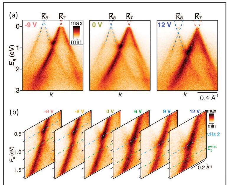
Influence of the gate voltage on the band structure. (a) Influence of gate voltage on the Dirac cone positions and (b) the position of the van Hove singularity. Adapted and cropped from original.
