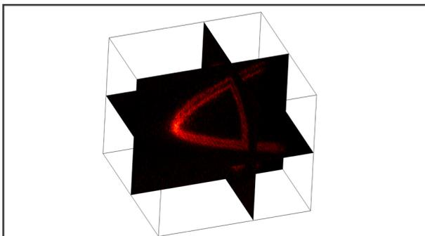
**Figure 1:** 3D representation of the ARPES data set measured with the DA30-L ARPES mapping mode and the VUV5k UV source. The complete data cube was measured in 10 min.
