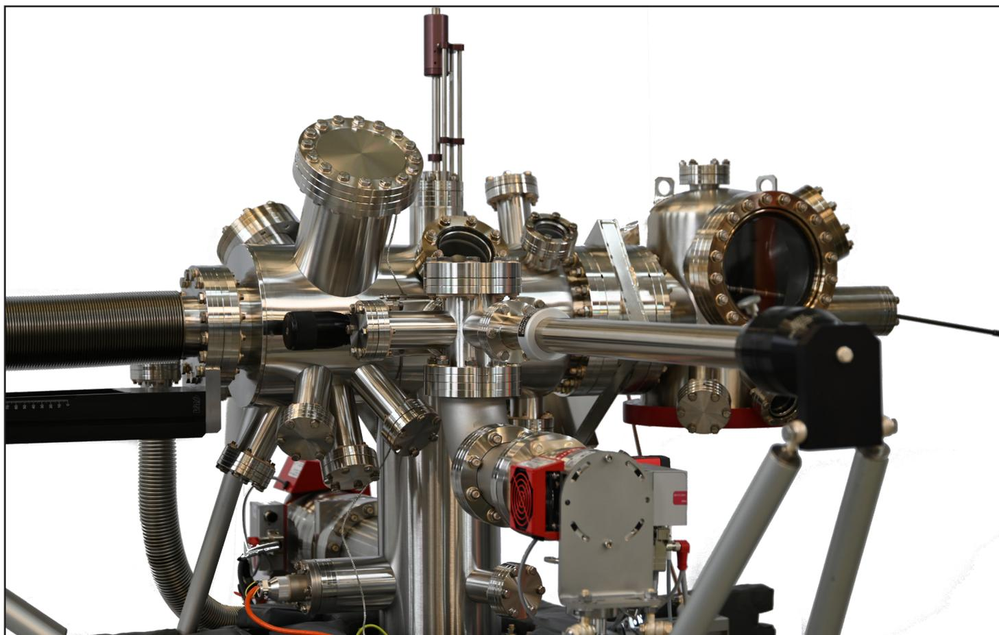
Scienta Omicron's Multiprobe Prep with ports for LEED and a set of 3 DN40CF ports for evaporators underneath. The chamber is extended with a separately pumped SPM bolt-on chamber and a loadlock chamber with a dedicated turbo pump.
