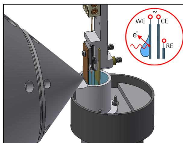
Figure 2: Analyser front-cone and dip & pull set-up using a three electrode system with working electrode (WE), counter electrode (CE) and reference electrode (RE).
