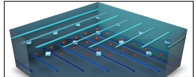
Figure 2: The proposed 2D surface code architecture consisting of three functional layers. The target dimensions are marked in the figure, with the qubits (red) and single electron transistors (squares) in the middle layer addressed by control lines vertically placed in separated places above and below the qubit plane.
