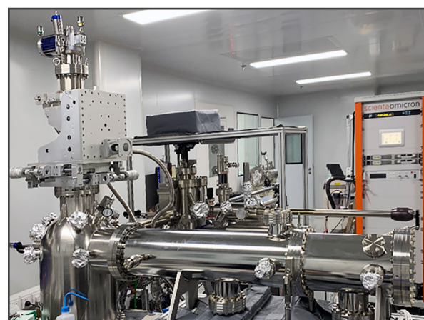
Figure 3. 2020 installation of an ARTOF Lab equipped with the ARTOF-2 analyser and a 5 axis closed cycle manipulator. An UHV transfer connects the ARTOF Lab with the Lab10 module for thin film deposition seen in the background.
