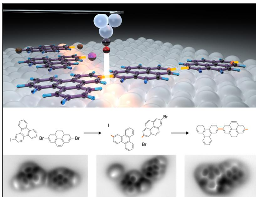
Figure 1: Constructing covalent organic nanoarchitectures via scanning probe manipulation. The halogenated precursors are adsorbed on an inert NaCl surface, which ensures their alignment in the plane but keeps them movable. The AFM tip is used as a “finger” for inducing the subsequent reaction steps by short voltage pulses. The activated and newly formed chemical bonds are shown in orange.
