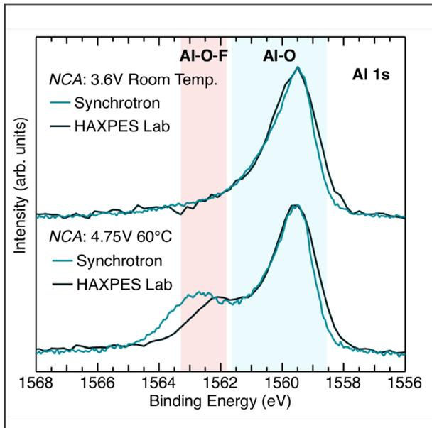
Figure 1: HAXPES measurements of the Al 1s for commercial  $\text{LiNi}_{0.8}\text{Co}_{0.15}\text{Al}_{0.05}\text{O}_2$  electrodes using both synchrotron (beamline I09 at the Diamond Light Source in UK, 6 keV) and HAXPES Lab (9.25 keV). Data reproduced from Ref.2
