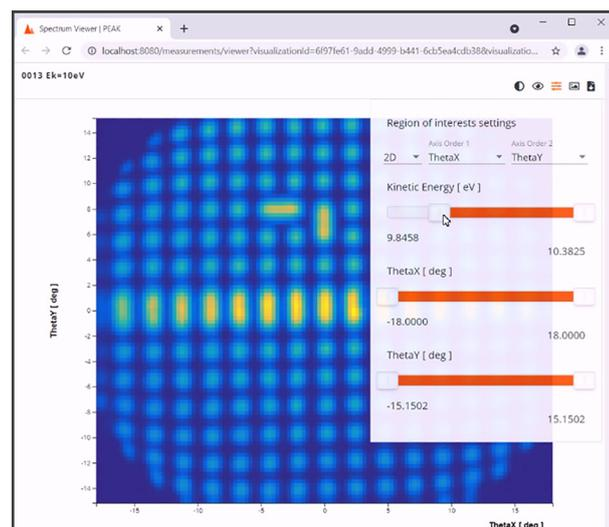
**Figure 1:** Data visualisation is done on the fly and can be applied to a selected slice or the complete data range. The visualised data is continuously updated as the measurement progresses allowing to explore data without interfering with the acquisition.
