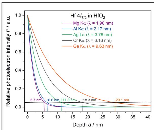
Figure 2: Relative photoelectron intensity  $P$  as a function of depth  $d$  for the  $\text{Hf } 4f_{7/2}$  core level in  $\text{HfO}_2$  using available laboratory X-ray sources<sup>1</sup>. The legend gives the inelastic mean free paths  $\lambda$  for  $\text{Hf } 4f_{7/2}$  at different excitation energies.
