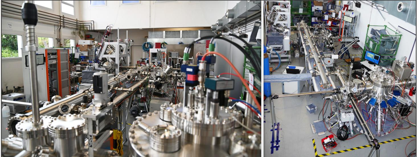
The new Ultra-High Vacuum (UHV) Materials Innovation Platform (MIP) combines a PRO-75 MBE for thin-film synthesis, a NanoESCA module for band structure and chemical analysis, and a Multiprobe Prep module with VT SPM for surface morphology studies. All modules are interconnected by a Linear Transfer Line (LTL). Photos from the factory in Taunusstein during the final acceptance test.
