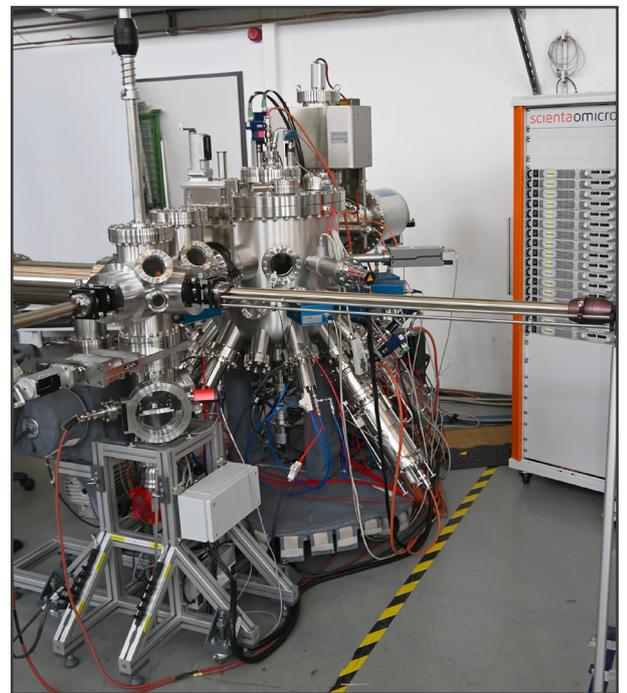
PRO-75 MBE configured for chalcogenide growth with cryopump and ion pump. The deposition chamber is designed to allow homogeneous epitaxial growth on samples up to the size of a 3inch wafer. A dedicated load lock is used to introduce 3inch carriers. Flagstyle sample holders can be separated from the 3inch carrier and transferred in-situ to the NanoESCA and VT SPM modules via the LTL.
