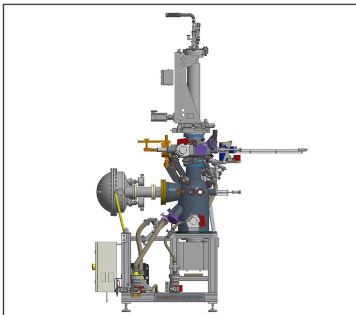
ARPES Lab: drawing generated by CREATE platform
