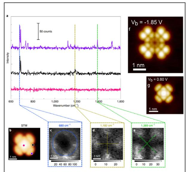
**High Resolution STM and TERS measurements with sub-molecular TERS contrast on a single CuNc molecule.**
