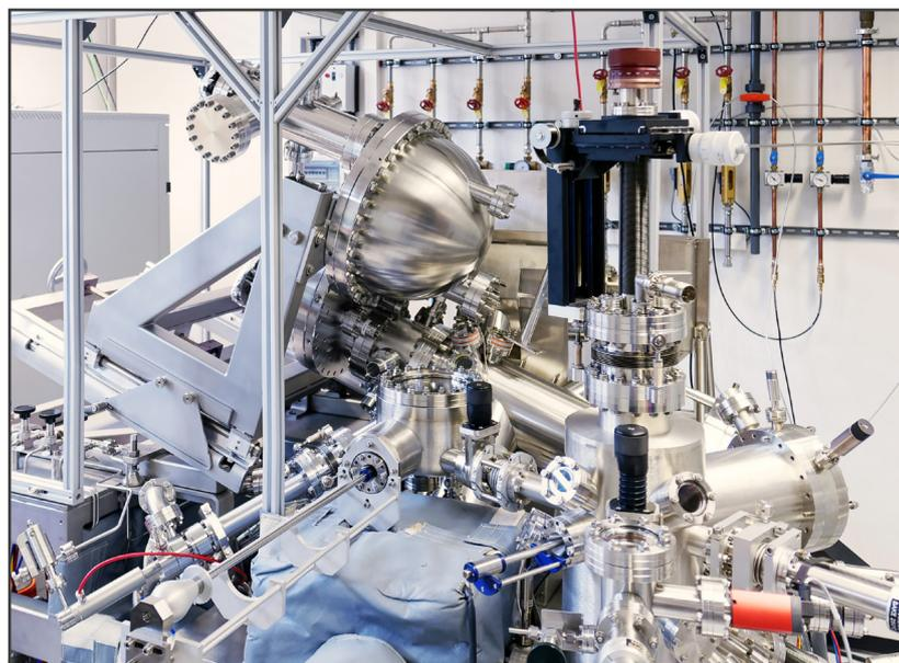
Figure 2: The NanoESCA installation at the MPI für Festkörperforschung (Stuttgart), group of Prof. Ulrich Starke [1]. The NanoESCA system is equipped with a preparation chamber, a HIS 14 VUV source, a monochromated X-ray source and a LHe cooled 4 axis manipulator.
