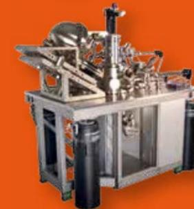
LT NANOPROBE UHV system with an extended XP type preparation chamber and two fast entry load locks. It features a UHV Gemini column for high resolution SEM, QPlus AFM functionality, a MATRIX SPM control system and a retractable NanoSAM energy analyser for Scanning Auger Microscopy and elemental mapping.
