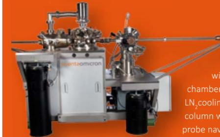
This LT NANOPROBE UHV system is designed for direct connection to a transfer line and is equipped with a horizontal XP type preparation chamber, and a separate manipulator for LN<sub>2</sub> cooling and heating. An Orsay Vortex SEM column with better 40nm resolution is used for probe navigation.
