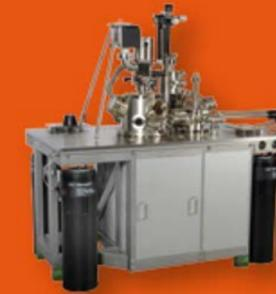
LT NANOPROBE UHV system with preparation chamber and Orsay e-CLIPSE SEM column, MATRIX SPM control system, a single fast entry load lock, QPlus AFM provision, and an additional optical port for laser excitation. The system configuration includes a separate preparation chamber with ports for sample sputtering, thin film evaporation, and a sample manipulator for heating up to 900°C.
