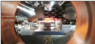
Advanced in-situ photoelectron experiments are enabled by virtually live snapshot data acquisition and extended sample manipulation possibilities, e.g. a wide temperature range (130 < T < 1100 K).
