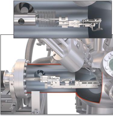
Cross-sectional view of the XPS-Lab illustrating two sample handling concepts. The Large Sample Carrier allows for mounting multiple samples and offers great flexibility for size and shape of sample specimen.
