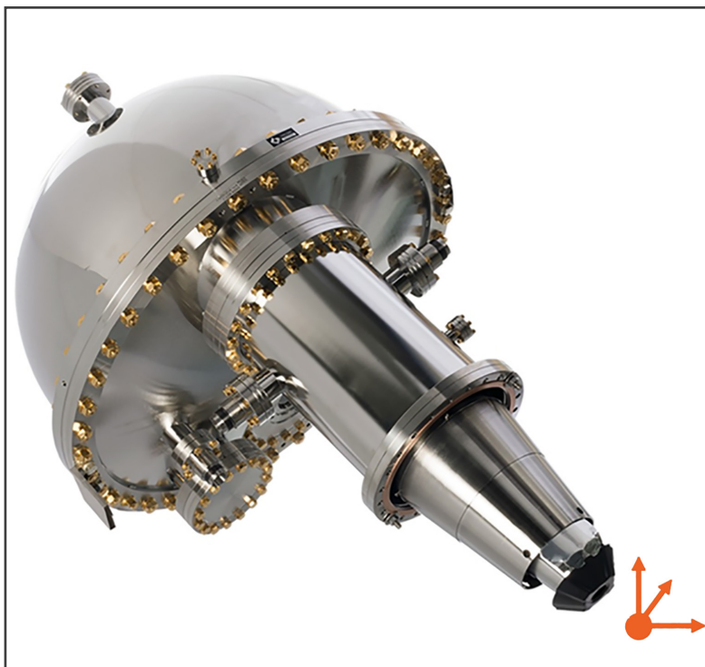
Figure 1: The DFS30, the new standard for angle resolved photoelectron spectroscopy, is equipped with Electrostatic 3D Focus Adjustment. Real time calculated lens tables allow to adjust and shift the analyser focal point to the emission spot on the sample, ideal for small spot \mu ARPES measurements.
