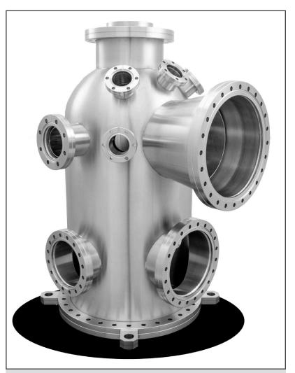
Chamber for an ARPES setup with UV laser source. It is based on the configurable chamber with ports configured to individual customer requirement. The double mu-metal liner provides best magnetic shielding for ARPES measurements at low kinetic energies and highest energy resolutions. The setup is completed by the research group with components for sample handling, light source, analyser, and vacuum system.
