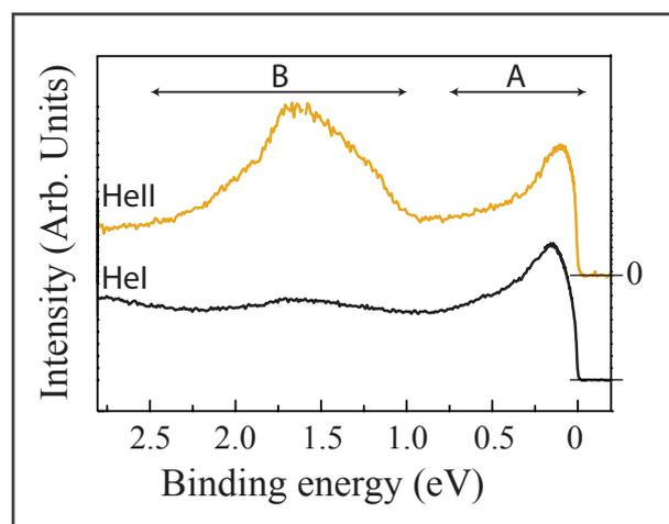
Figure 1: Valence band of the  $\text{EuFe}_2\text{As}_2$  compound recorded with Hel (21.2 eV) and HeII (40.8 eV) light. Two distinct features, denoted A and B can be identified for the spectra.
