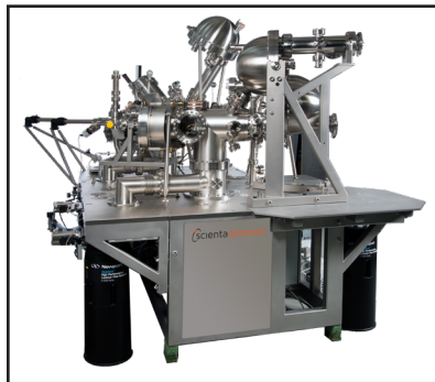
NanoESCA system equipped with vibration damping system, LHe cooled manipulator, HIS 14 VUV light-source and preparation chamber with pre-analysis capabilities.
